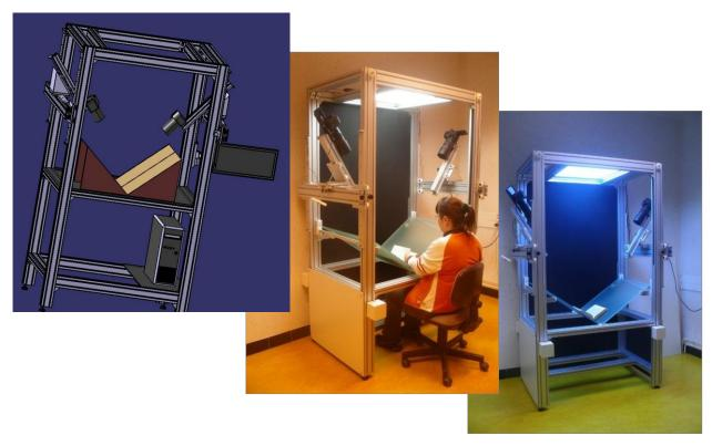
Figure 7. Self-made V-shape book scanner based on double EOS600D (18MPix each) developed by the French partner IFMA, CAD-Model and prototype
