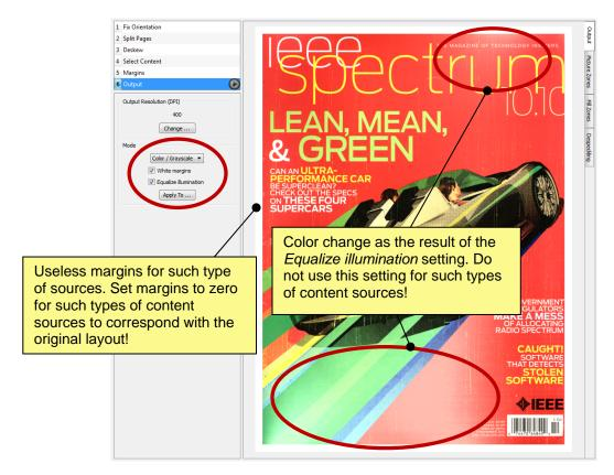
Figure B5 - All-over imprinted source type with 5 mm margin in each direction; colour mode settings see figure.
